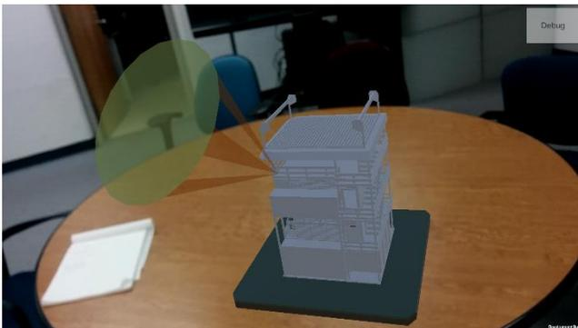
**Figure 6. A view frustum inspired by the Parafrustum. This geometric construct represents the exact angle and direction of the partner's perspective.**
