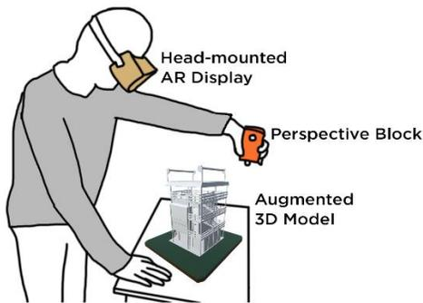
Figure 2. The Perspective Block concept.
